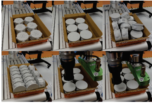
Figure 3 Proposed scenarios for the robotic gripper evaluation
