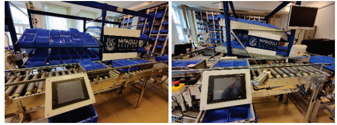
Figure 7 Placement and connection of two new HMI panels in the laboratory (self-made photo)
