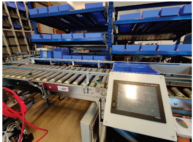
Figure 8 HMI panel serving roller track system after relocation (self-made)
