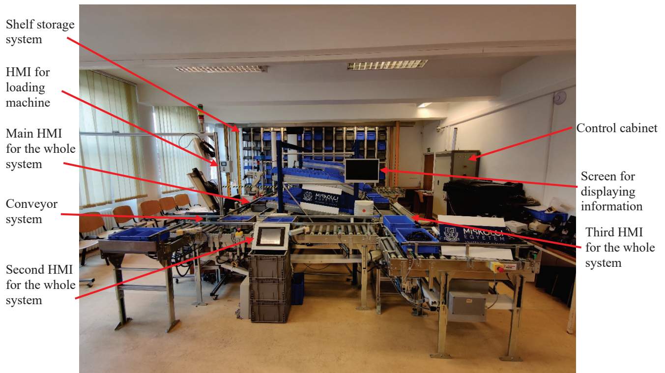
Figure 11 Logistics 4.0 laboratory at University of Miskolc in 2023 after development (self-made photo)
